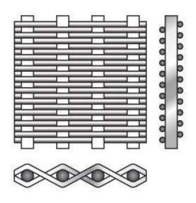
**Plain Dutch:** Primarily used as a filter cloth. The openings slant diagonally through the cloth and can not be seen by looking directly at the cloth. This weave has a coarser mesh and wire in the shute direction, giving a very compact, firm mesh with great strength.
