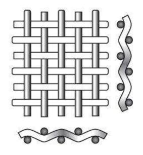
Twill Square: Each warp and shute is woven alternately over two and under two warp wires. This gives the appearance of parallel diagonal lines, allowing it to be used with heavier wires with a particular mesh count (that is possible with the plain weave wire cloth). This ability allows the applications of this wire cloth to be used for greater loads and finer filtration.
