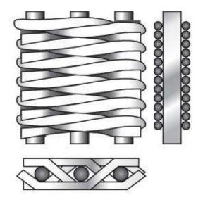
Reverse Plain Dutch: A filter cloth in which the larger count of wires is found in the warp and the smaller count in the shute, thus reversing the method used in plain and twilled Dutch weaves. The warp wires have a smaller diameter than the shute wires and touch each other, while the heavier shute wires are woven as tightly together as possible.
